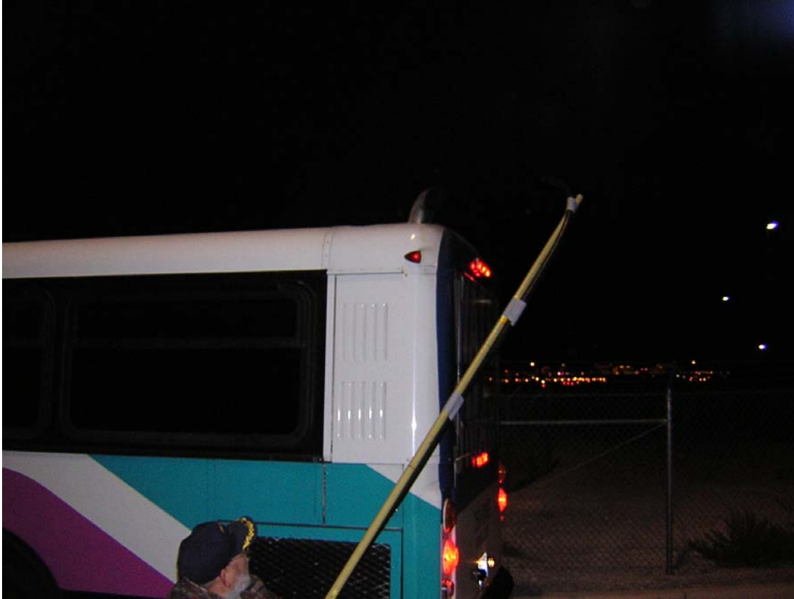
Figure 2-4. Sampling of on-road diesel vehicles at RTC bus depot, Las Vegas, NV.
