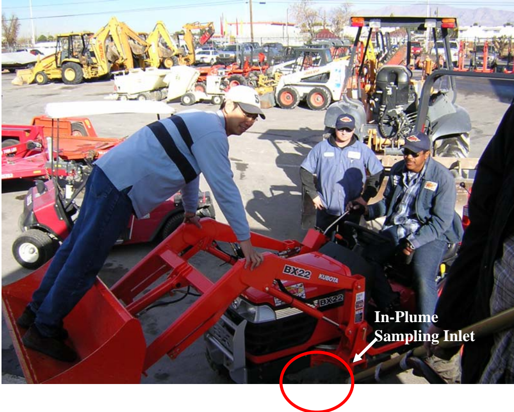
Figure 2-5. Non-road diesel engines mimic field operation by (a) lifting a power generator and (b) lifting a weight of 160 pounds. (Circle indicates sample collection point.)
